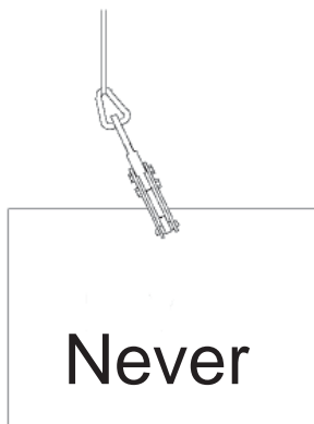
Figure 5: Always position the clamp in line with the sling.
